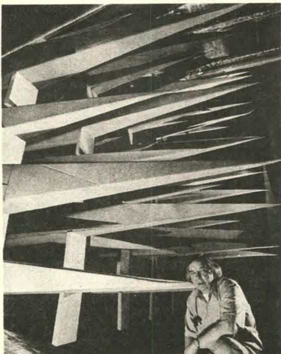
JIM REED with some of the RF absorber cones in EMES. Jim conceived the idea of a building that is essentially a coaxial transmission line.
