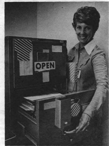
NEW SECURITY DEVICES remind Eve Baughman (4010) that safe drawers are open. The sign and the striped device are easy to spot; the flag springing to verticality is less visible but it's there—note blur.
