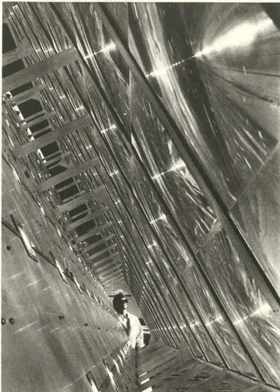
CONCENTRATED sunshine is viewed by Gene Hammons (5132) in this system that includes 135 plastic Fresnel lenses (right) focusing upon an equal number of silicon solar cells at left. Electrical output of cells is increased about 50 times using concentrated light.
