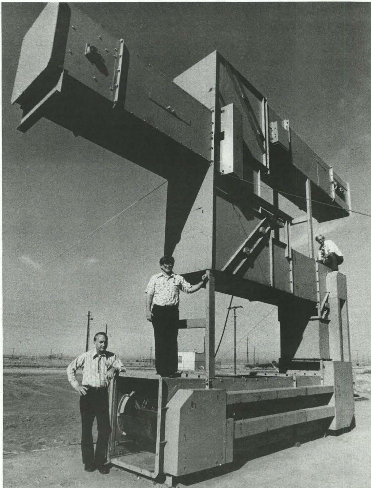
SLUDGE CONVEYOR will be one of the principal elements of pilot facility in which sludge will be irradiated to eliminate pathogens. Aim is to produce material suitable for use as a fertilizer or soil conditioner. From Beneficial Uses Program Division 5445, Jack Sivinski, Marvin Morris and Jim Pierce stand with machine.
