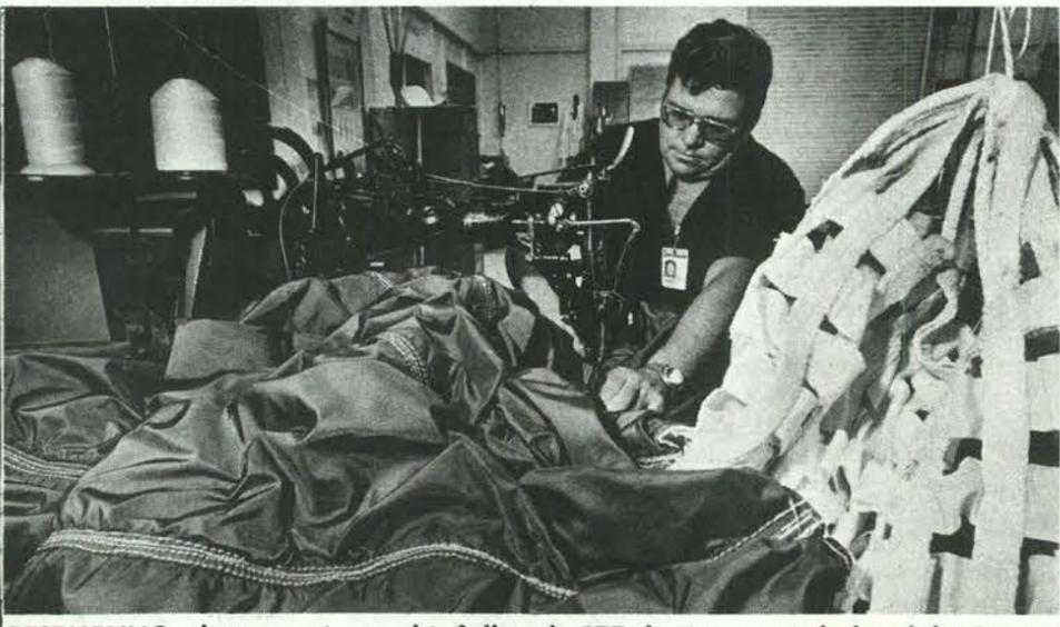
**RESEMBLING** a huge petticoat, this full scale B77 chute is grappled with by Dennis Cronin as he sews lifting liner onto canopy. Largest chute handled in Lab measured 36 feet in diameter.
