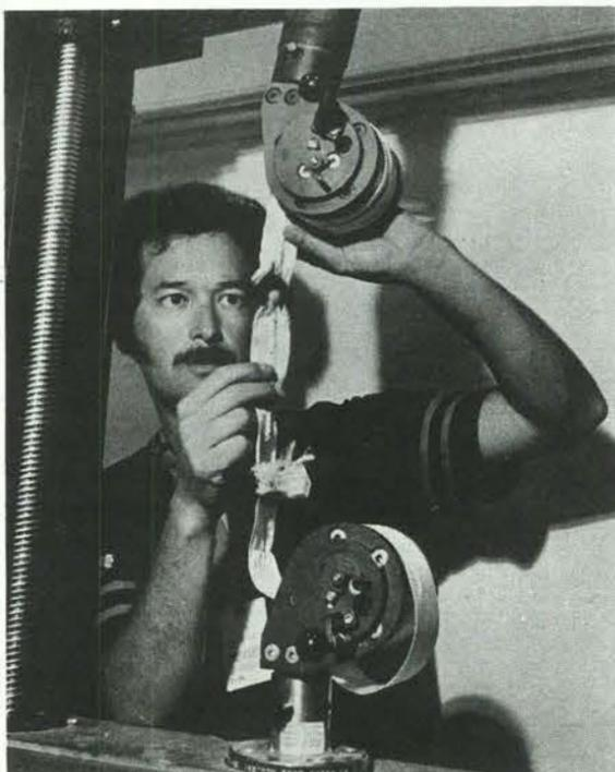
**BREAKING POINT** of parachute material is determined on this machine by Ken Ronquillo. Goal in chute development is maximum strength, minimum volume because space available is always limited.
