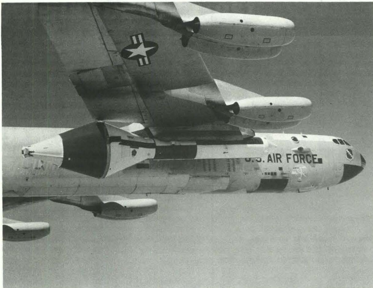
TEST VEHICLE for the space shuttle parachute system hangs on wing of B-52 mothership. Note slot in wing flap to accommodate aft section (which contains the recovery system). Sandia is serving as a consultant to NASA for the recovery system development program.
