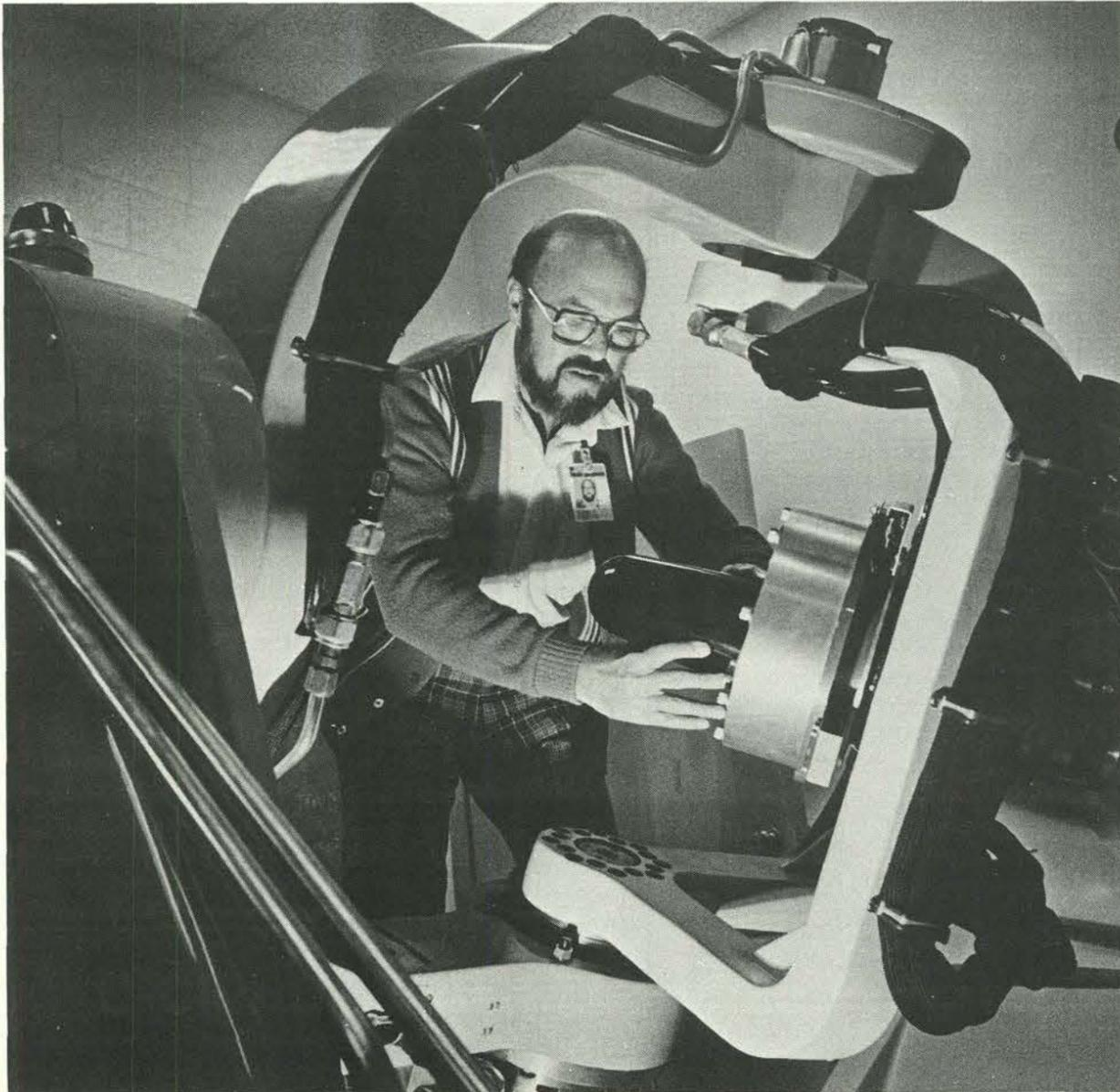
FLOYD FORSYTHE (1336) attaches a prototype guidance system module to the three-axis angular motion simulator in Sandia's Flight Simulation Laboratory. The simulator generates the angular rates of momentum expected in flight.
