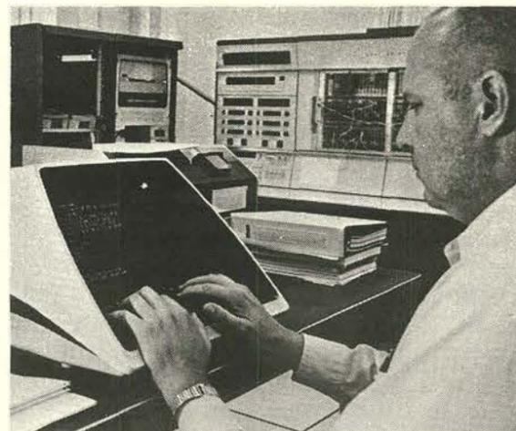
HYBRID COMPUTER in Sandia's Flight Simulation Laboratory is a useful tool in component design. John Phelan (1321) is working on the design of an autopilot for the guidance and control system of the Extended Range Bomb (ERB).
