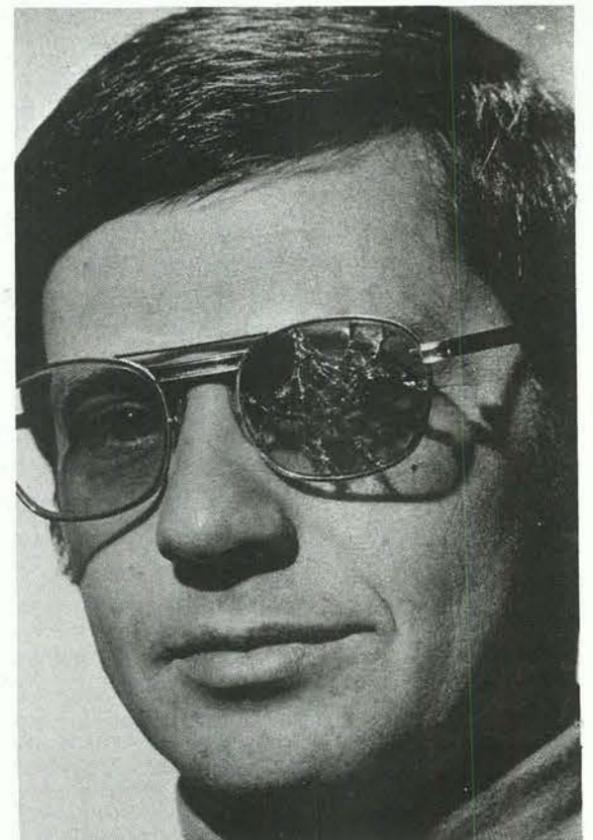
**KER-CHUNK &/OR SPLATT!** So went Ward Bower's safety lens as he applied his skill-saw to a piece of lumber. Whirling blade threw chunk of wood into lens in spite of guard. The lens broke but Ward's eye was untouched, converting ordinary citizen Ward Bower (2167) into Wise Owl Ward Bower—a member of that group whose vision has been saved through use of safety glasses.
