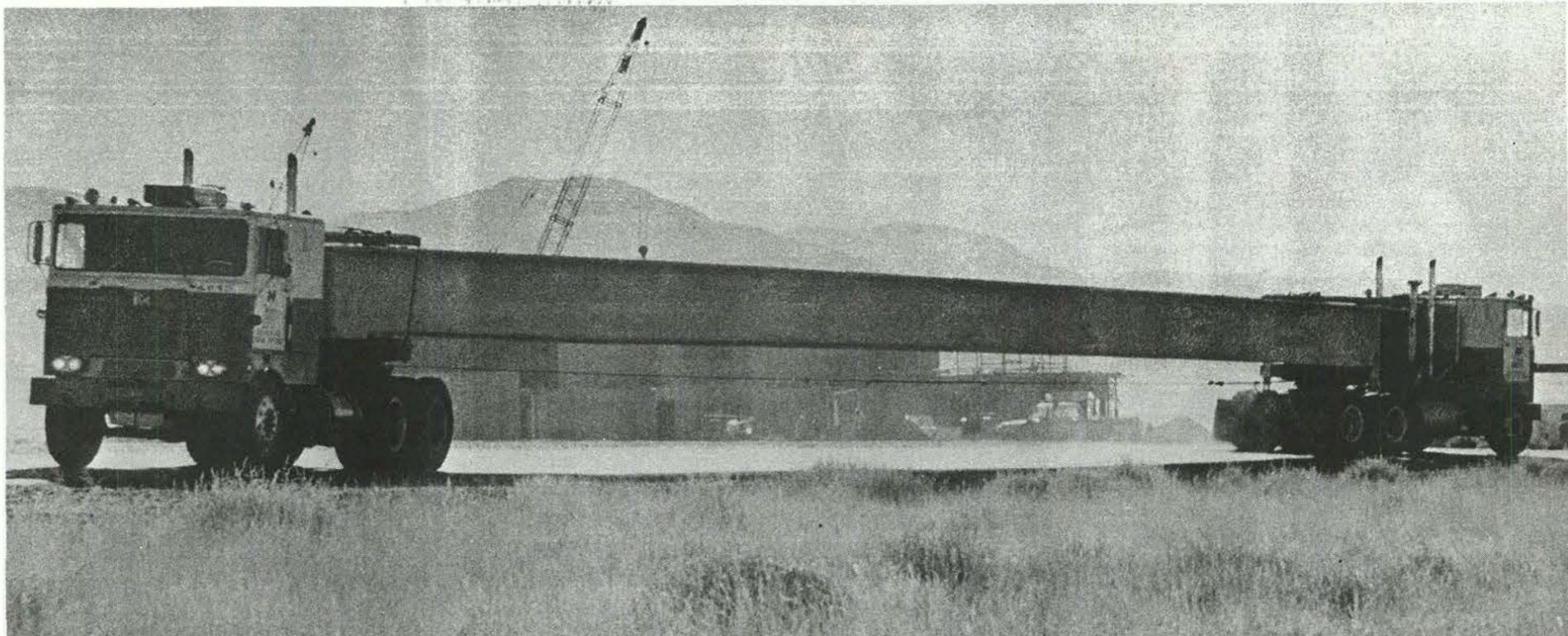
**FULL SPEED AHEAD?** To demonstrate the adage that two heads are better than one, this strange looking rig is used to transport the huge concrete T-beams that form the roof of Sandia's new Electron Beam Fusion Facility (scheduled for completion in Fall 1978). The T-beams weigh 37 tons and are 128 ft. long. With both tractors in place, the total length from bumper-to-bumper is 150 ft.—a formidable vehicle to encounter on the freeway. Manufactured locally, the
