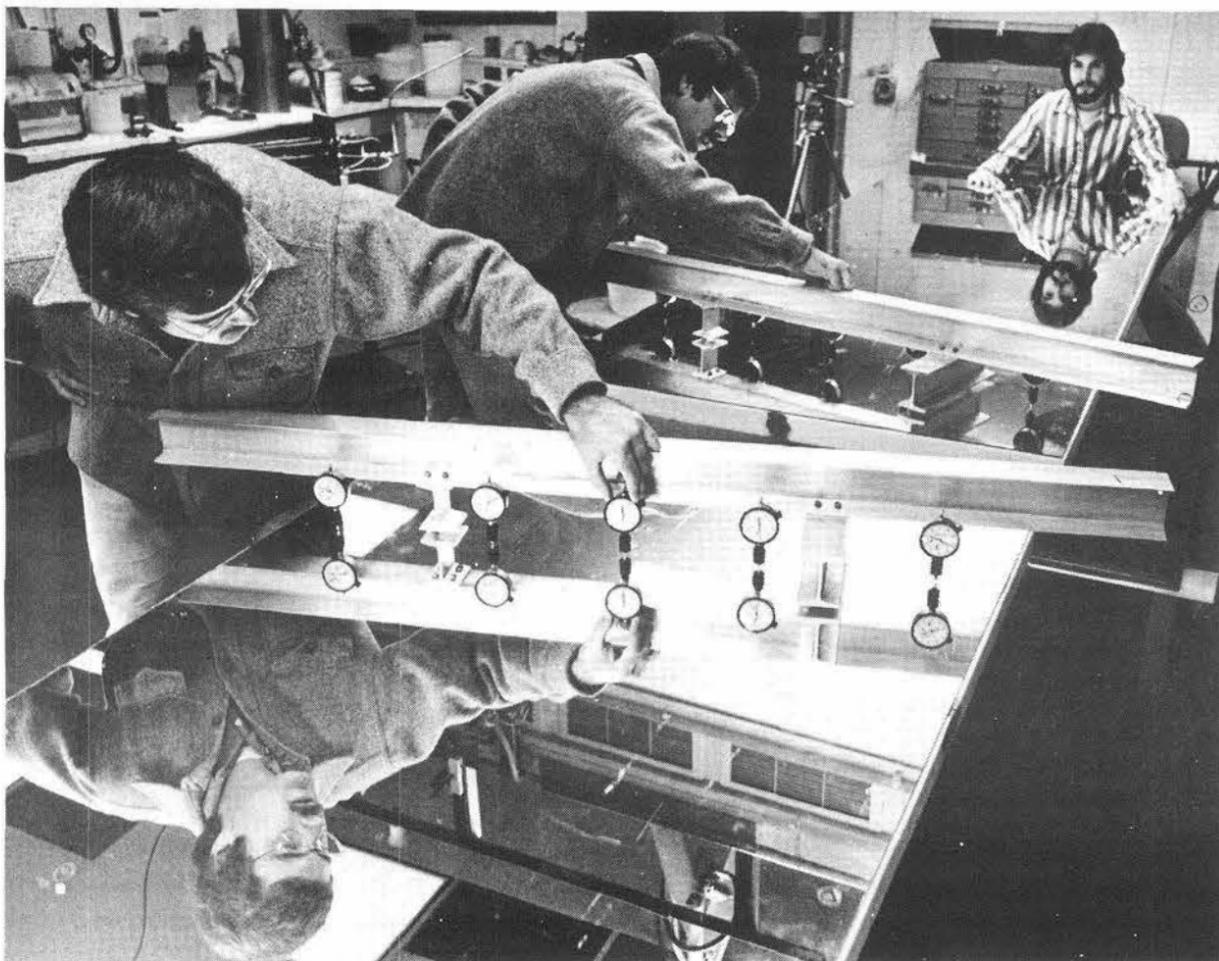
SEEING DOUBLE—Bill Delameter (foreground, 8121) and Dale Boehme (8424) check out mirrors Dale and others in the Plastics Lab have built to McDonnell-Douglas specifications. Here they're measuring deflections down to hundredths of a millimeter.
