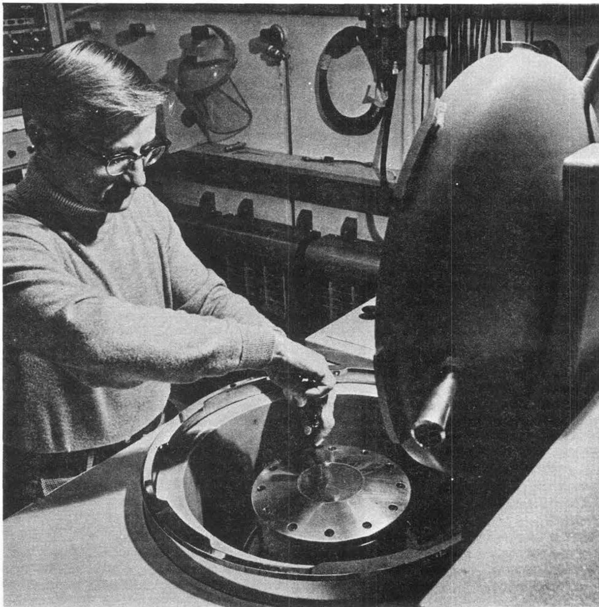
**JUST BEFORE THE EXPLOSION.** Jim Kannolt (2533), designer of a test system to simulate the high spin environment of a nuclear artillery shell, installs a rotor containing an exploding neutron generator. To compensate for initial and post-explosion imbalances, the rotor sits on a self-centering quill shaft. Plastic and metal foams inside the rotor mitigate shock and trap and hold shrapnel.
