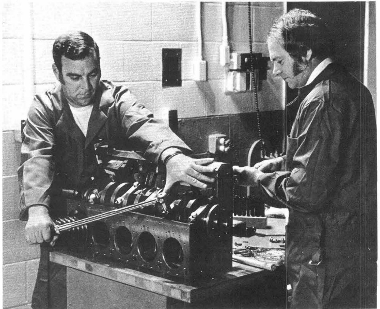
ASSEMBLING THE CRANKCASE of the Pouliot Variable Displacement Engine prototype are Dennis Sparger and Bill Kent (both 8352). SLL's work with the VDE is now complete.
