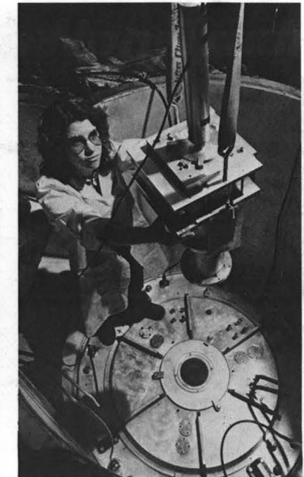
GINA NOACK (5244 - ESA) guides pin-hole camera into position for laser alignment on diode assembly of Proto I.
