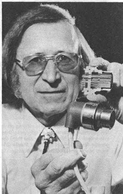
ED EHRMAN (2154), one of the principal developers of LAC, Lightning Arrestor Connector, shows internal weapon cabling and cutaway of the LAC. If lightning zapped weapon through external skin connector, the LAC would short out on surface of conducting web and current would go to case ground—thus protecting internal components downstream from cabling.
