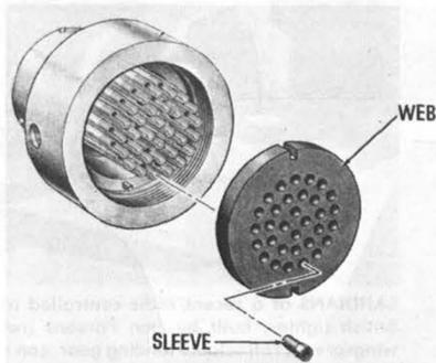
THIS EXPLODED VIEW of the Lightning Arrestor Connector shows conducting web and dielectric sleeve. The non-conducting sleeve crowds electric field into air gap between connector pin and conducting web. Breakdown arc partially vaporizes pin and web materials, causing a dead short which protects vital internal weapon components.
