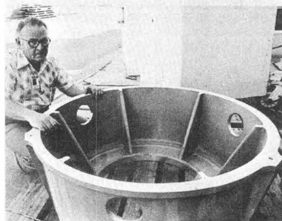
NOT EVERY DAY in this age of miniaturization of components does Sandia's foundry (org. 9573-5) perform pours of 1600 lbs. or more. Recently, however, the foundry poured 17 large tracking camera mounts for use with new instrumentation at Tonopah Test Range and White Sands. In top photo, left, C. B. Torres checks the packed sand mold. Top right is the pour. From overhead bridge cranes hang two ladles containing 800 lbs. of molten aluminum alloy
