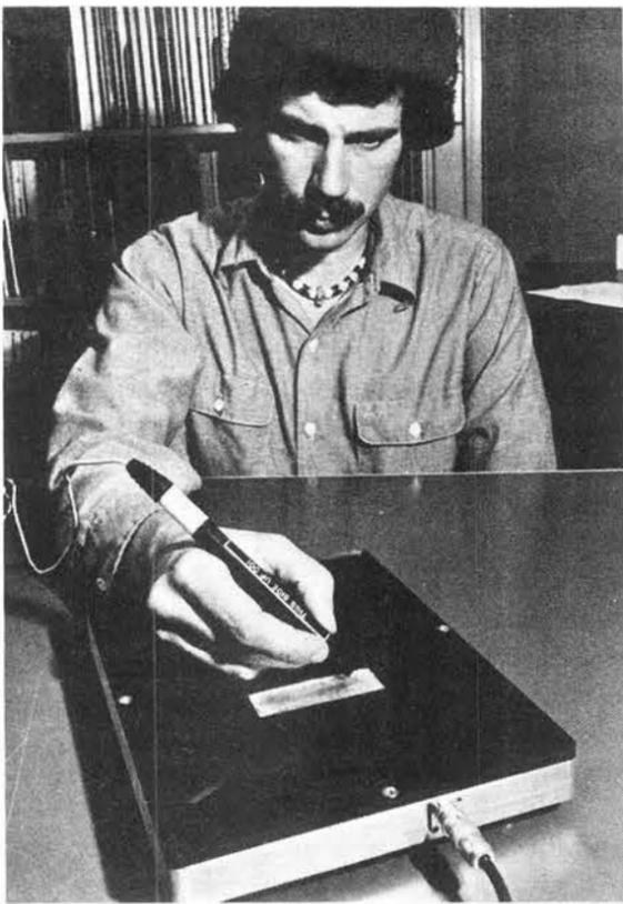
J. B. SNELLING (5133) demonstrates a recently-patented ballpoint pen and writing tablet which produces a unique electronic profile of an individual's handwriting. It could be used as part of a controlled access security system.
