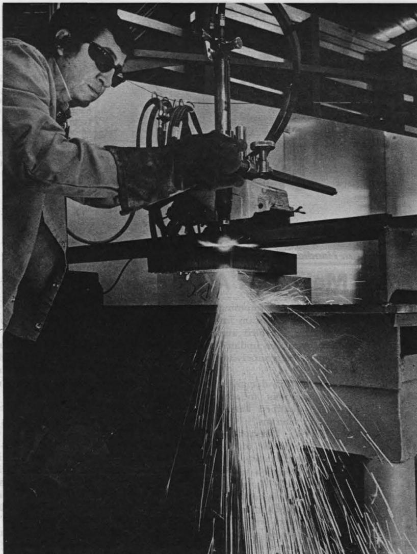
TORCHMAN George Lujan flame cuts metal billet. Metal stock up to six inches thick is available. Workers in raw stock warehouse all handle a variety of cutting tools.
