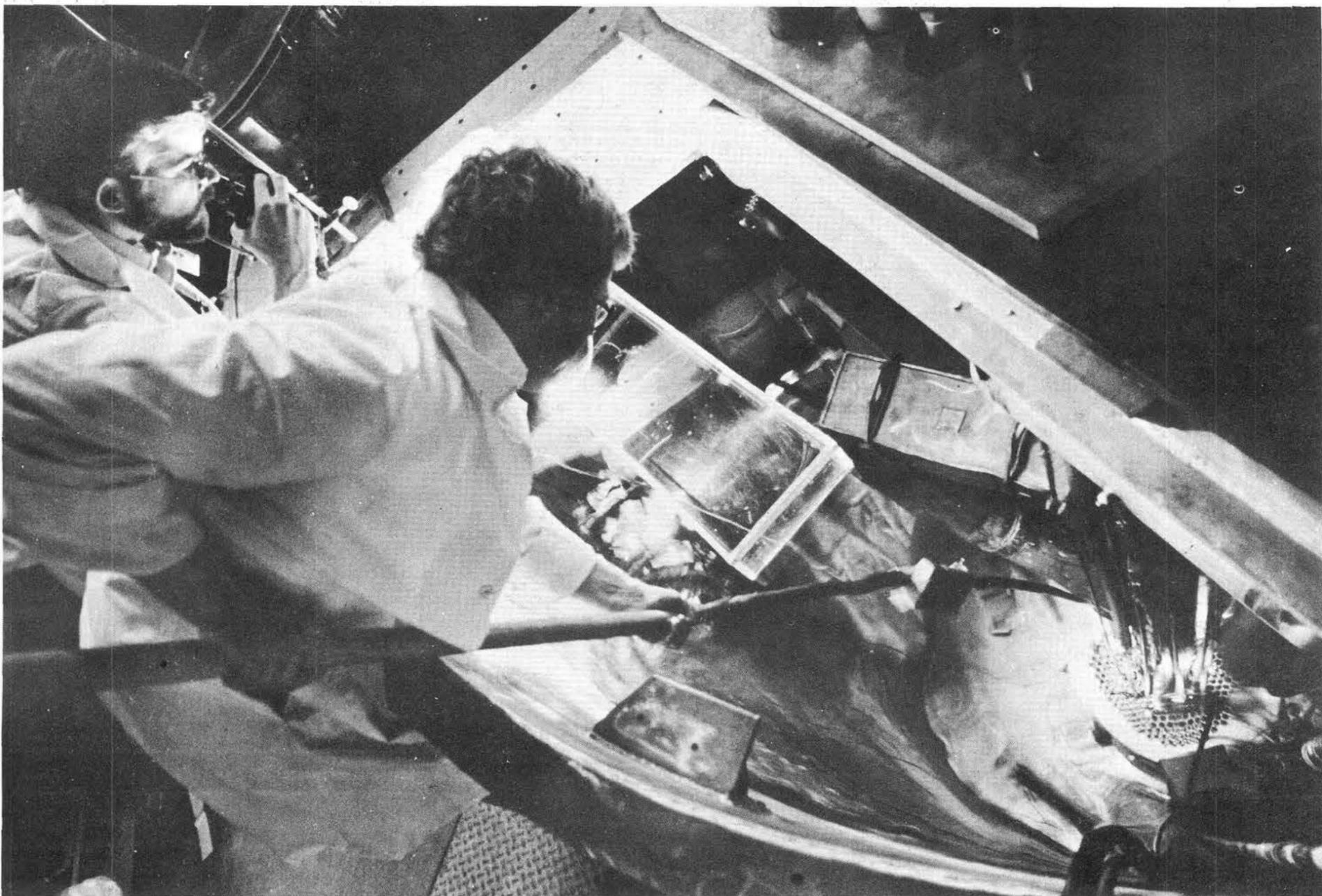
WORKING with a special tool, Ken Bolt (5451) inserts fuel rods into the ACPR core at the bottom of the 30-ft. shielding pool of water. Ted Schmidt (5451)
