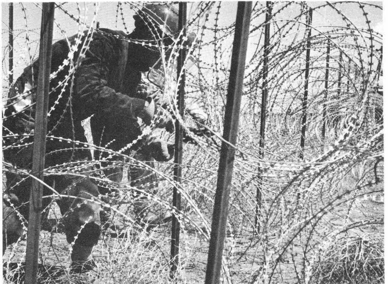
CONQUERING CONCERTINA WITH DETERMINED SHEARS. Two "aggressors" cut away at barbed tape entanglements with bolt cutters to establish how long it would take to breach such a barrier. *Barrier Technology Handbook*, just published by Org. 1711, contains data on this and wide variety of other barriers. See page 8 for story and photos.
