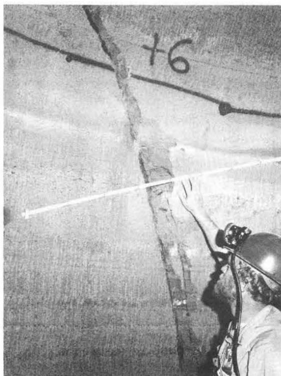
**BILL VOLLENDORF (1133)** examines a crack produced by hydraulic fracture experiment in the volcanic tuff of G-tunnel at NTS. Bill directs field operations for Sandia's Geophysical Laboratory at NTS.
