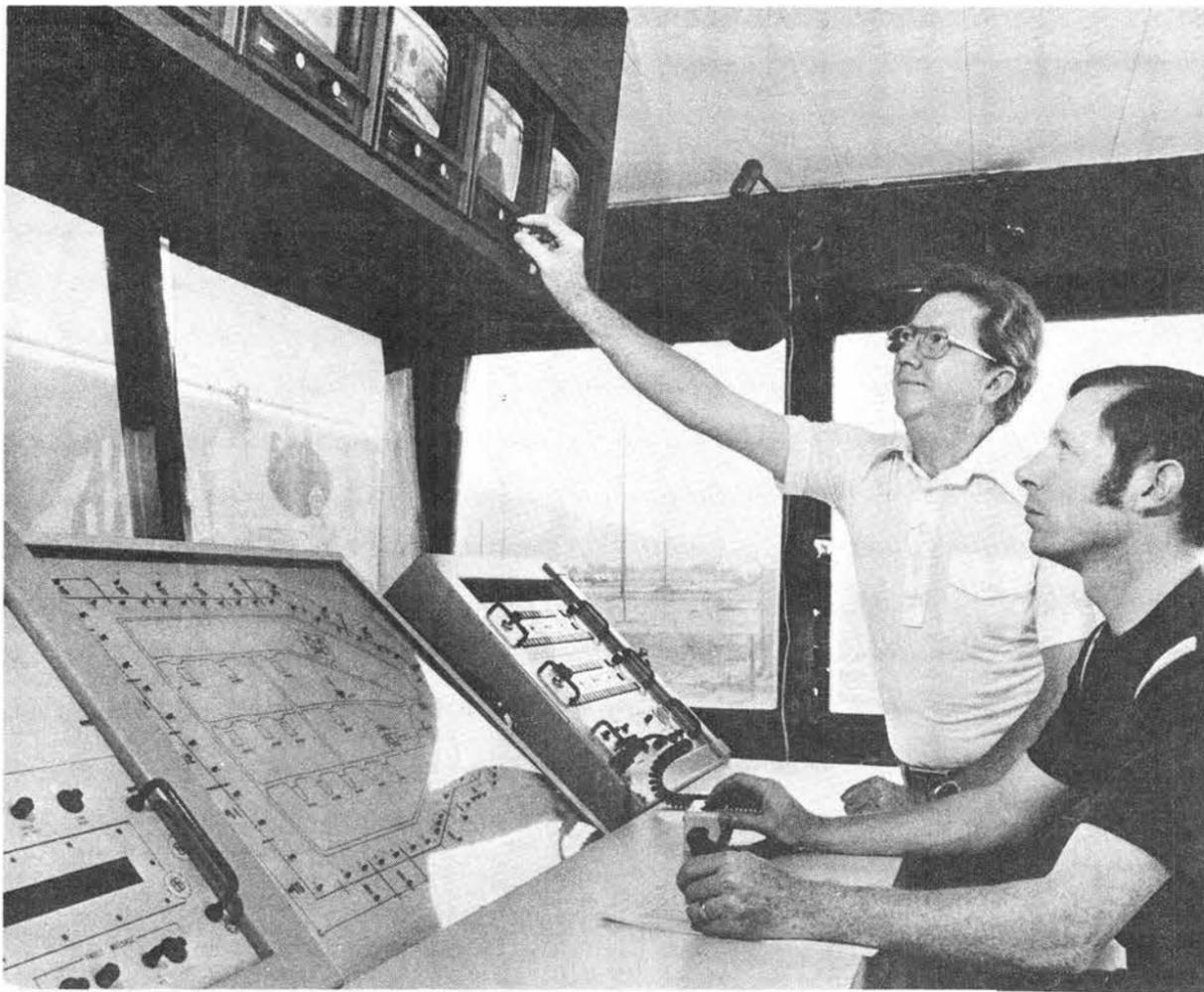
SYSTEM TEST of the Sandia developed Perimeter Surveillance System, Closed Circuit Television, is performed by Paul Stickler and Hovey Corbin (both 1733). They are at the Security Police operator's position in the control cab. In operational use, cab is positioned on a tower 30 to 50 ft. above the ground.
