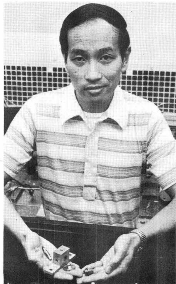
TO MEASURE THE BANG of an explosive actuator, Ray Ng assembles these parts: (left to right) a pressure transducer, a housing assembly, a slider, and the actuator being tested. Laser focused on the actuator during its explosion provides velocity information.
