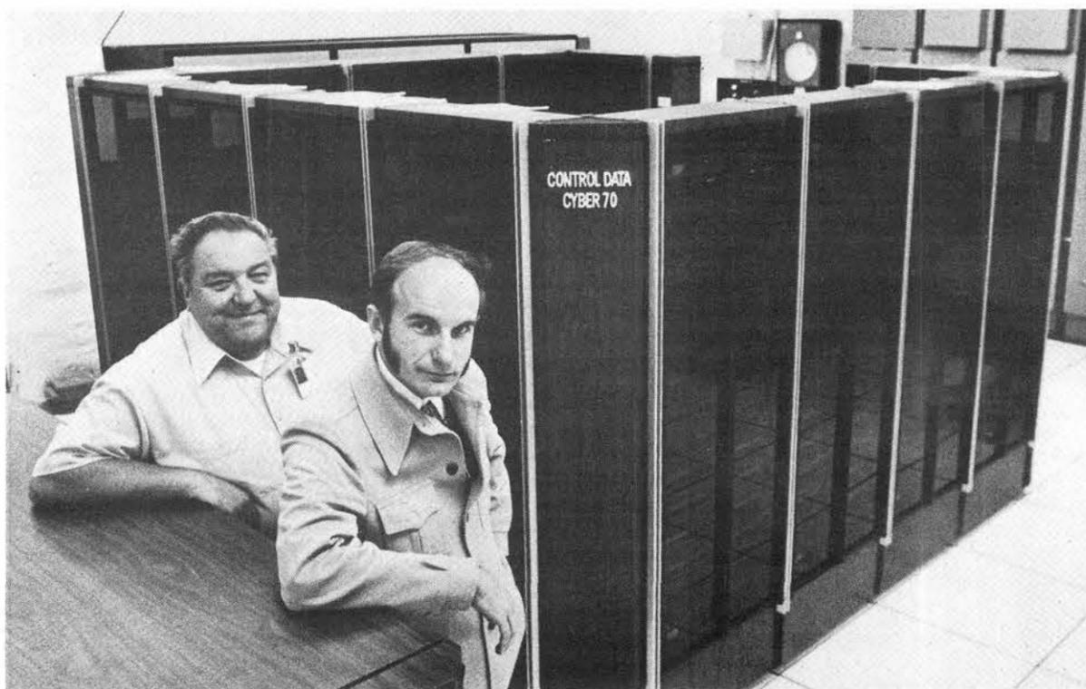
NEW COMPUTER — Now operational as part of Sandia's Scientific Computing Network is this Control Data Cyber 76. A Class IV machine, the new computer is faster and has a greater capacity than the CDC 6600 which it replaces. The Network now uses this machine, a CDC 7600, two CDC 6600's with extended core storage and various peripheral machines. Jack Westbrook (2631), left, directs operations of the Network; Paul Lemke (2641) supervises software.
