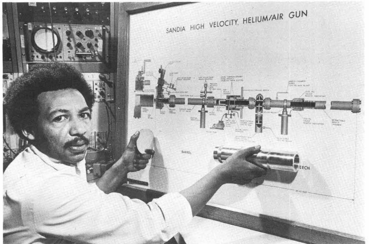
FAST GUN — And much used. In fact, shot number 1500 was fired off this month in Sandia's High Velocity Helium/Air Gun, now in its 16th year. G.T. Holman (5131) holds target and projectile. Compressed gas gun is used in shock-wave research.
