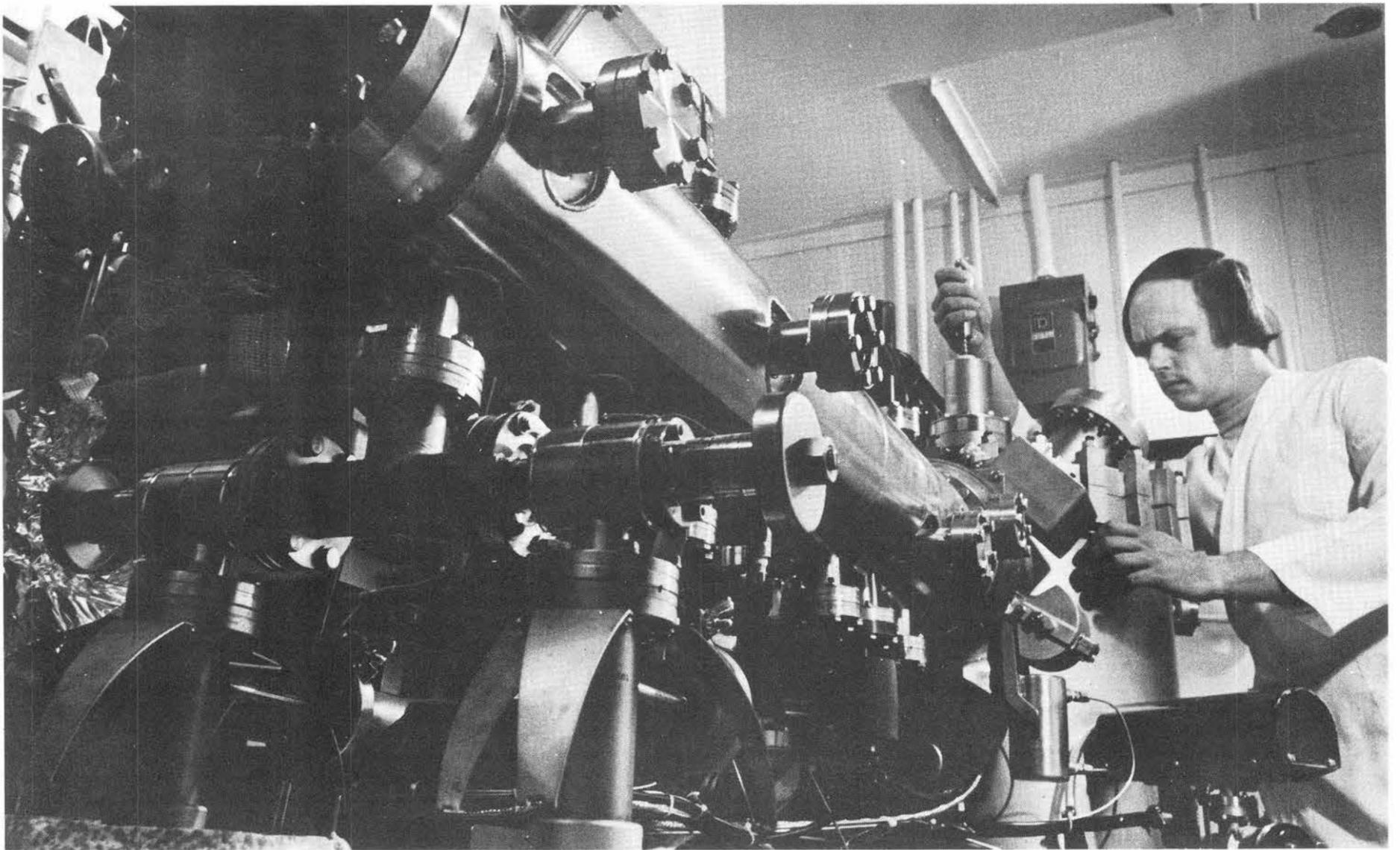
TERRY MASON, Development Lab Division 1472, transfers parts between the two sections of the evaporate load system, one portion of which is used for thin-film deposition, the other for deuterium or tritium gas loading.
