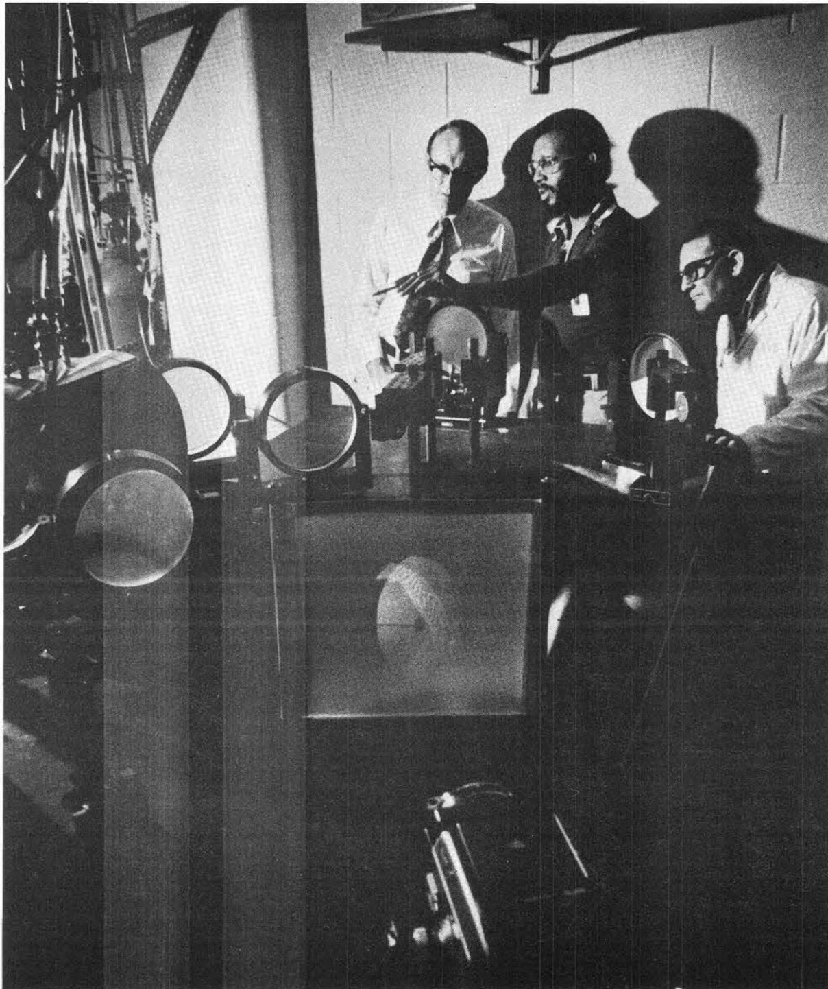
5500 DIRECTOR ORVAL JONES is briefed by Ron Boyd (5511) on studies being made to measure heat transfer coefficients in the annulus between a simulated radioactive fuel assembly and an outer cylindrical cask. Paul Montoya (5512) adjusts mirror that guides path of helium neon laser and projects image showing thermal activity on screen in center of picture.
