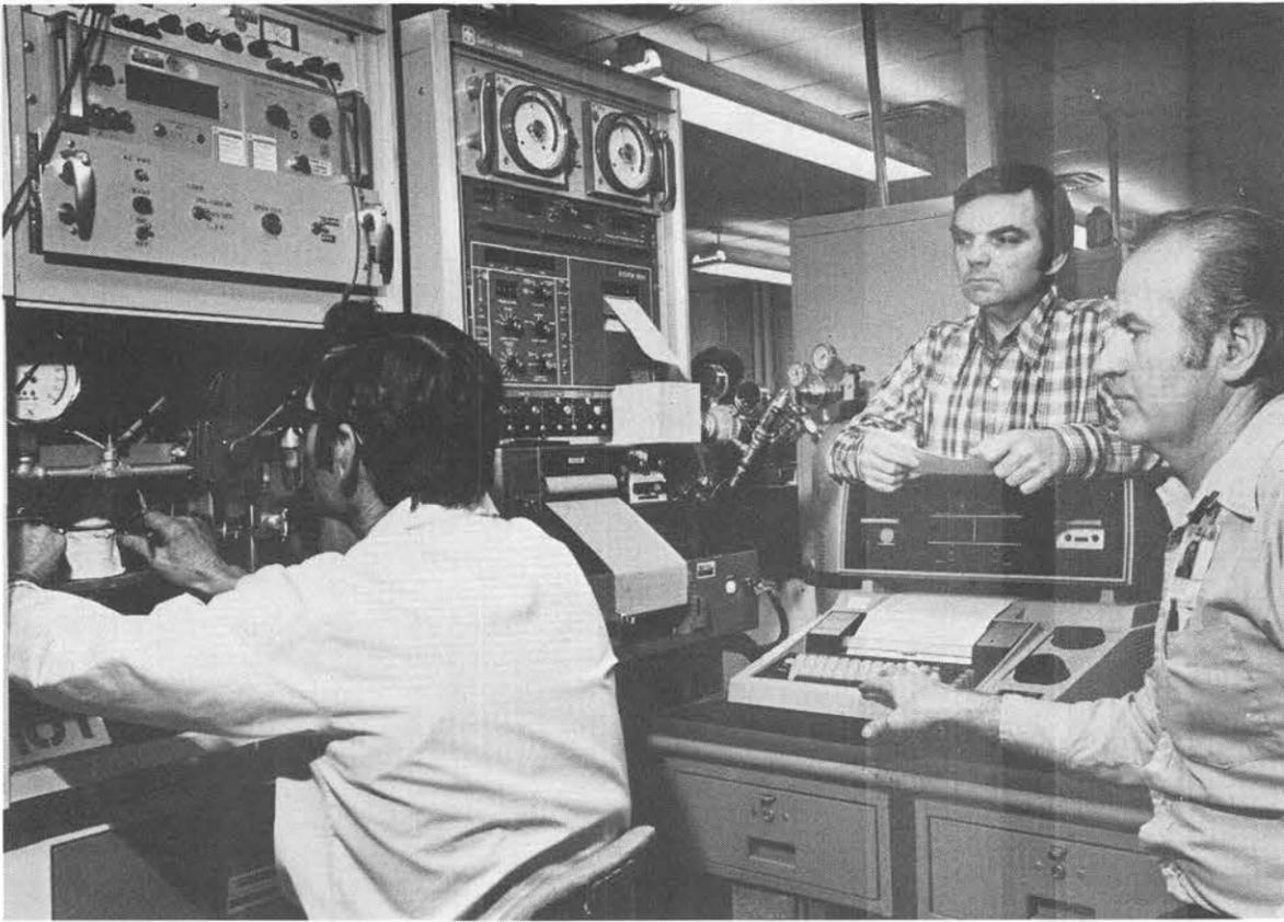
ROD QUINN (WHO HEADS EXPLORATORY BATTERIES DIVISION 2523) and Arlen Baldwin (right) watch Don Bush (also of 2523) as he places a single cell of an experimental thermal battery into an automatic tester. Tests measure electrochemical effectiveness of various anode/cathode/electrolyte combinations at variety of heats. Division is working on small, light, long-lived thermal batteries.
