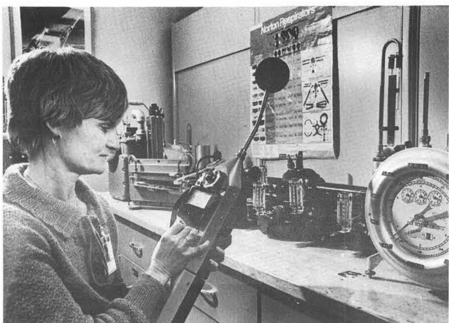
NOISE CAN BE A CONTAMINANT, TOO, and Joanne Pigg (3311) checks out a meter used to measure sound levels. This is one of dozens of special instruments used to measure concentrations and types of contaminants — one of many methods used to assure that Sandians have a safe work environment.
