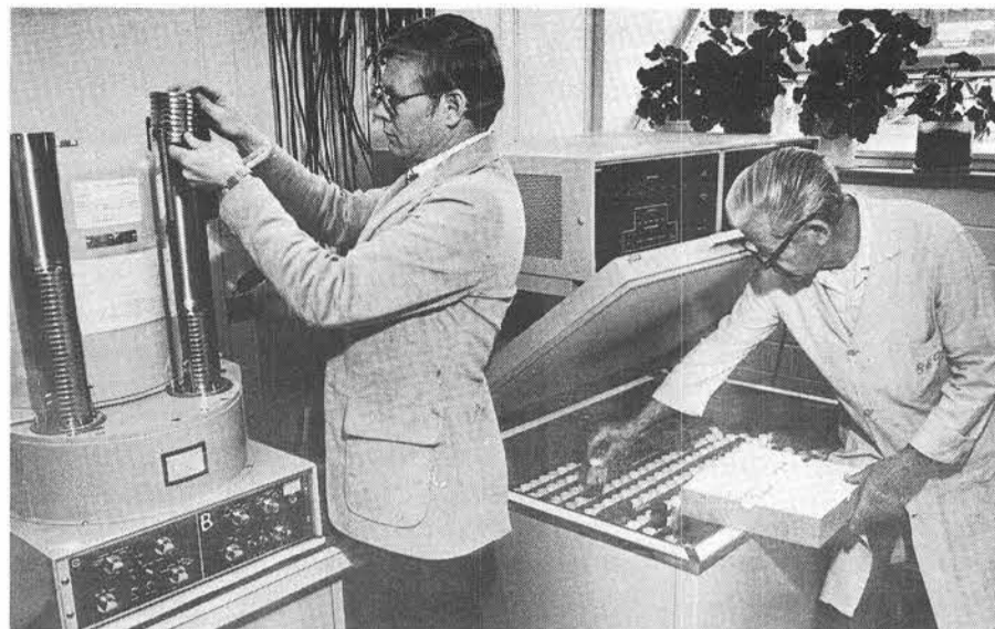
MEASURING RADIATION. Billy O'Neal, left, and Grover Edwards (3311) load samples into equipment which measures levels of radiation. Dry samples come from chem labs at Sandia, from swipes and smears taken by health physicists at various lab locations, and from soil samples. Liquids, tested in scintillation counter at right, are analyzed to make sure chemistry experiments stay within safe radiation limits. The equipment can also be used to identify unknown isotopes and their concentrations.
