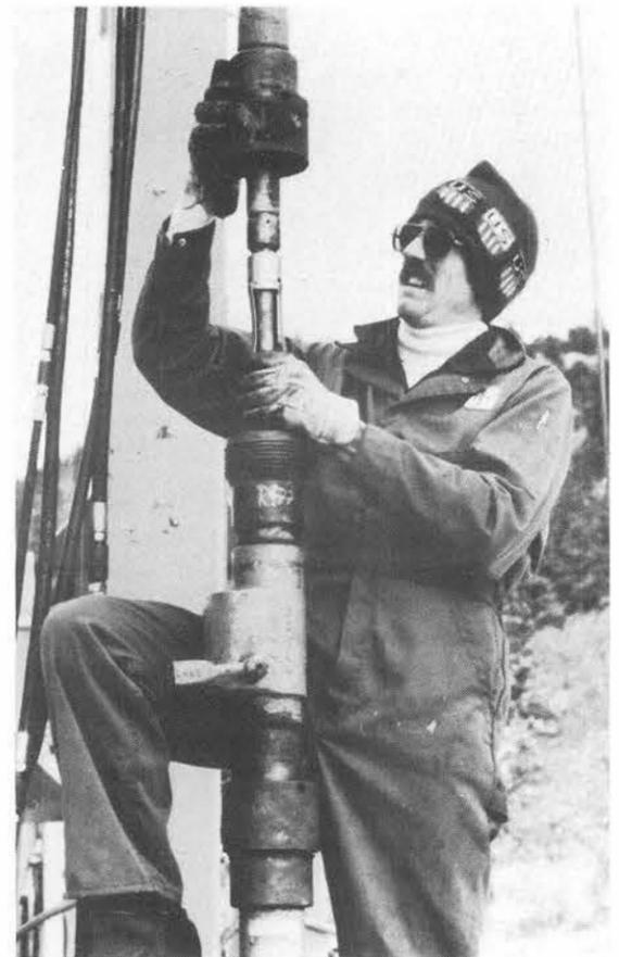
**HOW HOT?** — Joe Coquat of Geothermal Technology Division 4736 inserts a prototype of a high-temperature well logging tool into a Union Oil geothermal wellhead. Instrument passed first field test, operating at temperature of 275°C.
