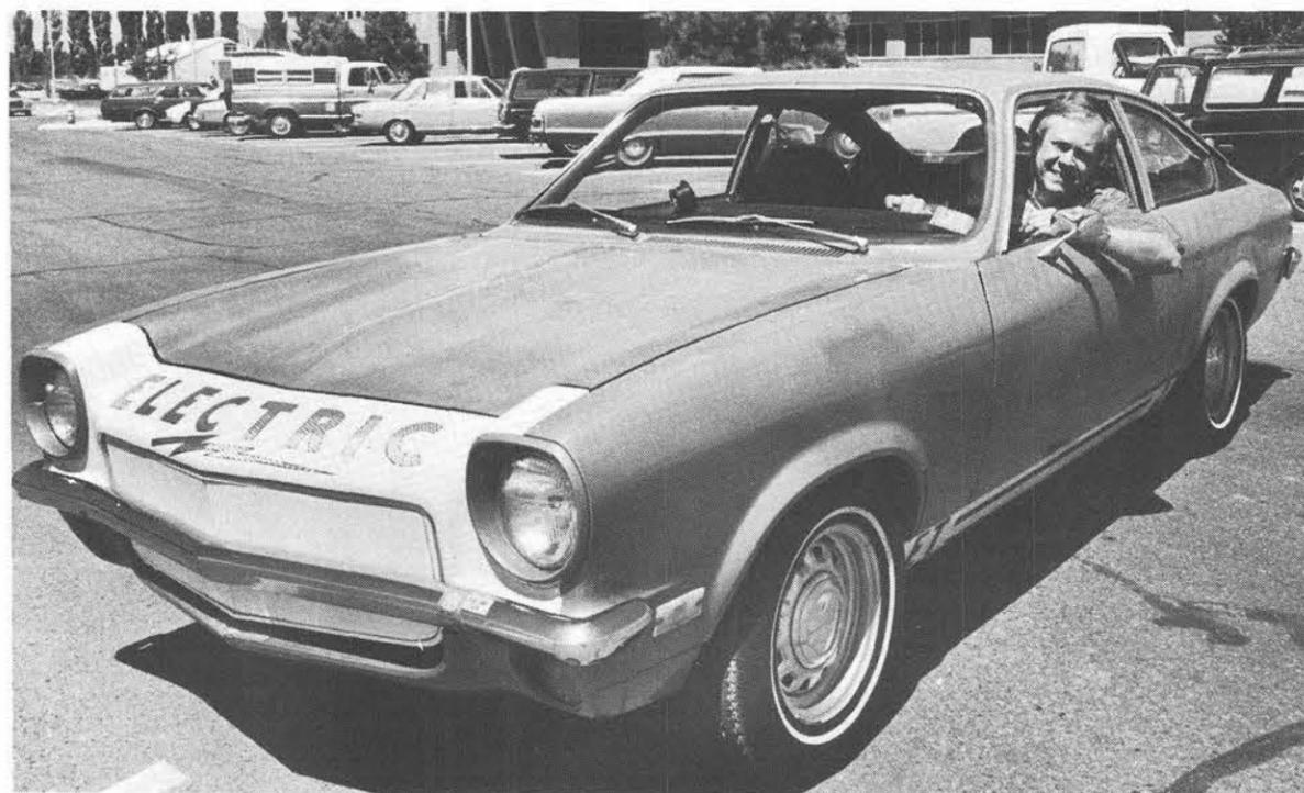
DICK BASSETT (2354) occasionally drives his home-built electric Vega to work (when he can talk his wife out of it). It's a high performance (60 mph with quick acceleration) vehicle with limited range (35 miles on a charge) and costs between 1¼ and 3 cents per mile, depending on fuel adjustments and electric rates.
