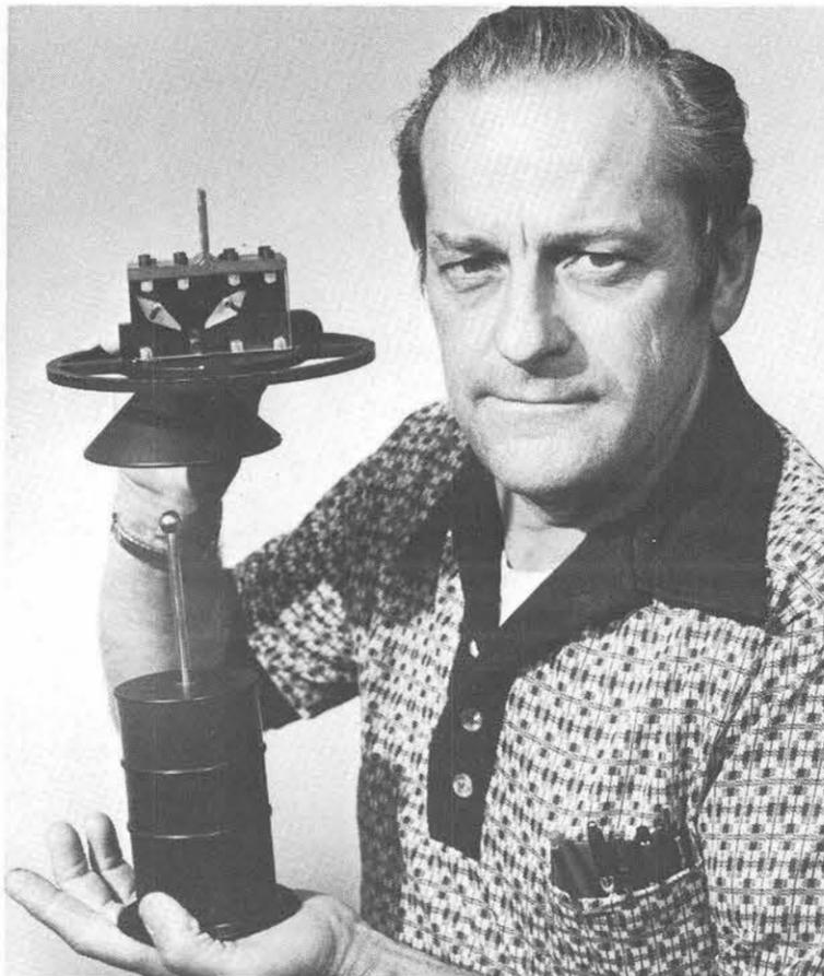
GENE ZUCUSKI (2323) displays a model of his "automatic hook." Hanging on the end of a single cable operating from a crane, the hook captures and releases ball-and-shaft-equipped containers simply and effectively. In plexiglass chamber above the guide ring, the capture and release levers are visible, the only moving parts within the device.
