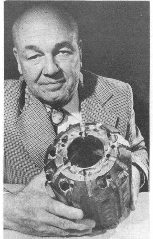
LEONARD BAKER of Drilling Technology Division 4741 and Sandia's pressure coring drill bit. In recent tests, the new bit performed significantly better than a conventional pressure coring bit.
