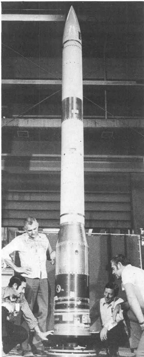
ROCKET PAYLOAD, 16.5 ft. in length and weighing 550 lbs., is checked for spin balance in the Mass Properties Lab in Bldg. 892 by Ted Krein (1525), standing, project leader; Ernie Niper (1525); Hovey Corbin (1525), and Harry Blechinger (1137). Two of the payloads will be launched into the shadow of a total eclipse off the coast of East Africa Feb. 16.
