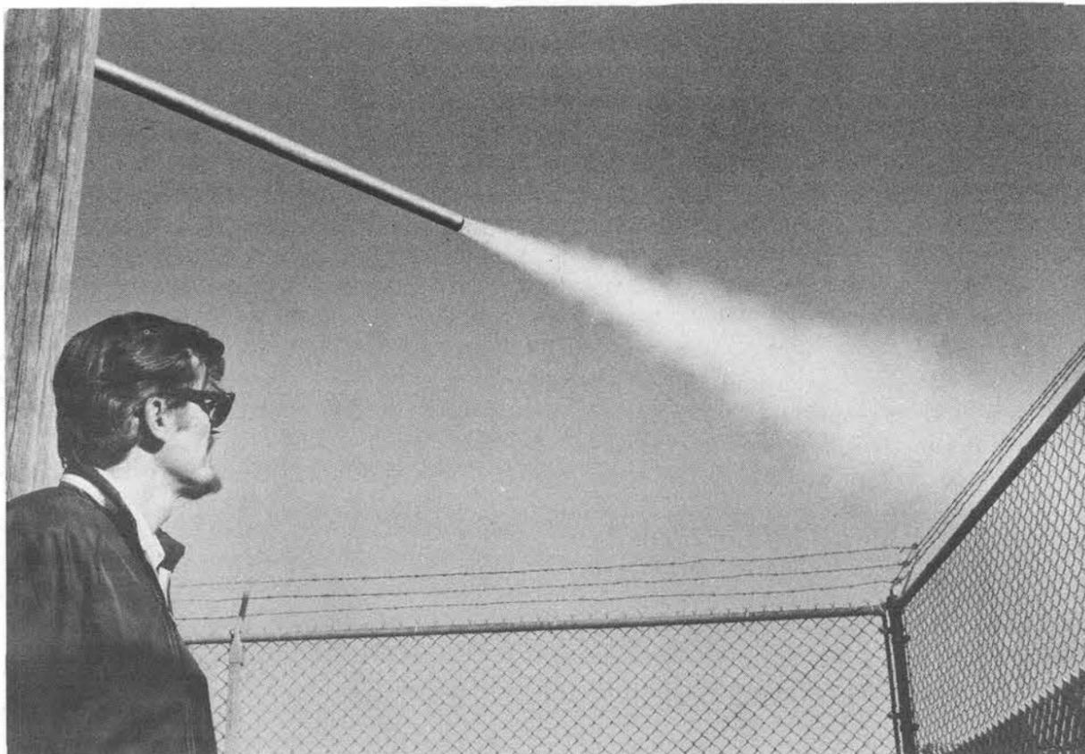
RON FOX, supervisor of Enhanced Oil Recovery Division 4738, watches operation of a prototype steam generator that is scheduled for field testing this month in an oil reservoir near Bakersfield, Calif. The unit is rated at 1.2 thermal megawatts and produces a steam volume of 1500 standard cubic feet per minute.
