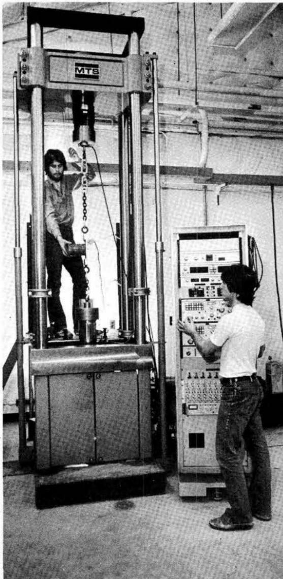
LARGE TEST FRAME in the Rock Mechanics Laboratory, Division 5532, applies either tension or compression loading up to 220,000 lbs. on rock samples. Jerry O'Brien and Chris Robertson ready the apparatus for a test. A larger machine with a million-lb. load capacity is ready for installation in the lab.
