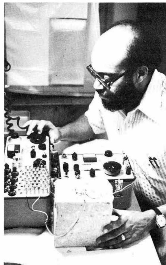
ADRIAN JONES measures residual stress in a tuff sample from the Nevada Test Site. Strain in the sample was measured, then overcured (circular cuts in the center of the block) and measured again by strain gages tied to the surface of the rock.
