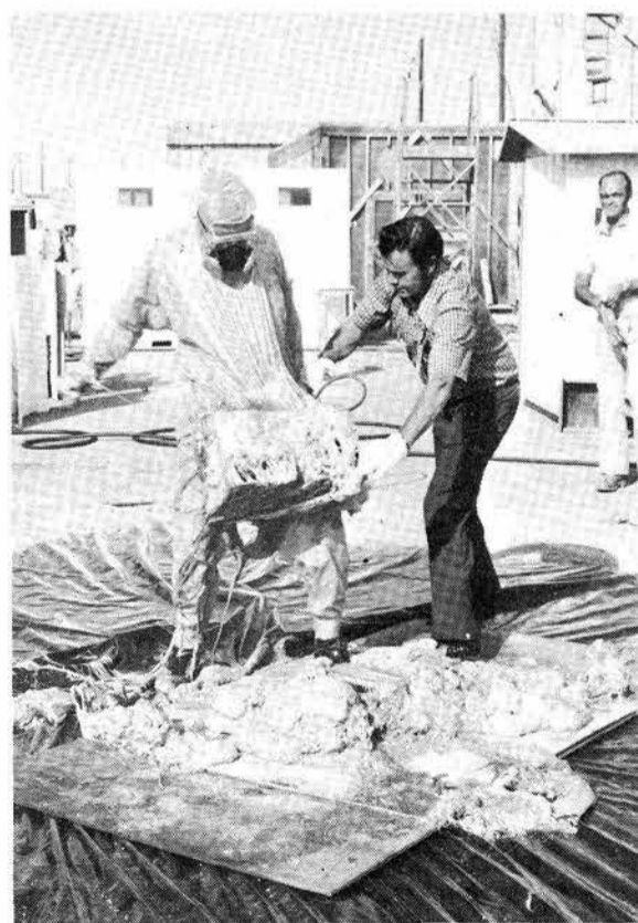
THE DIFFICULTY of movement while enmeshed in the sticky stuff is here demonstrated. An intruder has triggered the release of the foam, can barely move around, finally needs help in removing the canister stuck to his coveralls.
