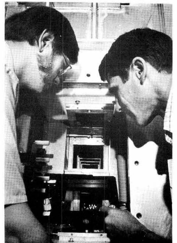
SCIENTISTS Terry Stalker and John Kelly (both 4426) ready CAIS for a reactor experiment. The 8000-lb. instrument must be raised from the 30-ft. deep reactor shielding pool to remove film after each experiment.
