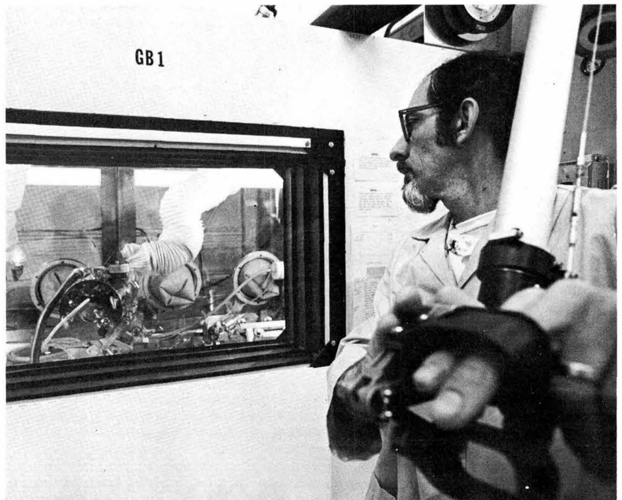
HOT CELL LAB supervisor Frank Gonzales uses manipulator to perform experiment with radioactive materials. Argon atmosphere in chamber behind eight-inch shielding window prevents atmospheric contamination.
