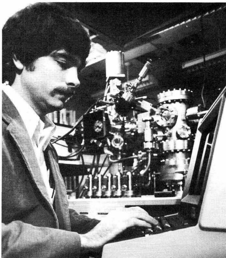
GARY KELLOGG (5114), co-developer of the pulsed-laser atom-probe, sends instructions to the computer that determines the chemical identity of atoms or molecules removed from the end of a sample shaped like a needle. The pulsed-laser technique opens new possibilities for studying surface catalytic reaction, the effects of ion bombardment of semiconductor materials and single atom and vacancy motion in atomic detail.
