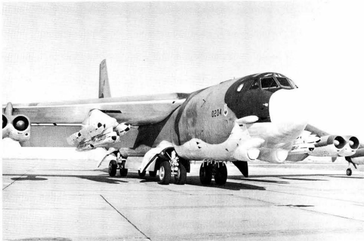
SIX AIR LAUNCHED CRUISE MISSILES, each armed with a Sandia W80 warhead, can be mounted under each wing of the B-52 aircraft. The ALCMs can also be carried internally in the B-52.
