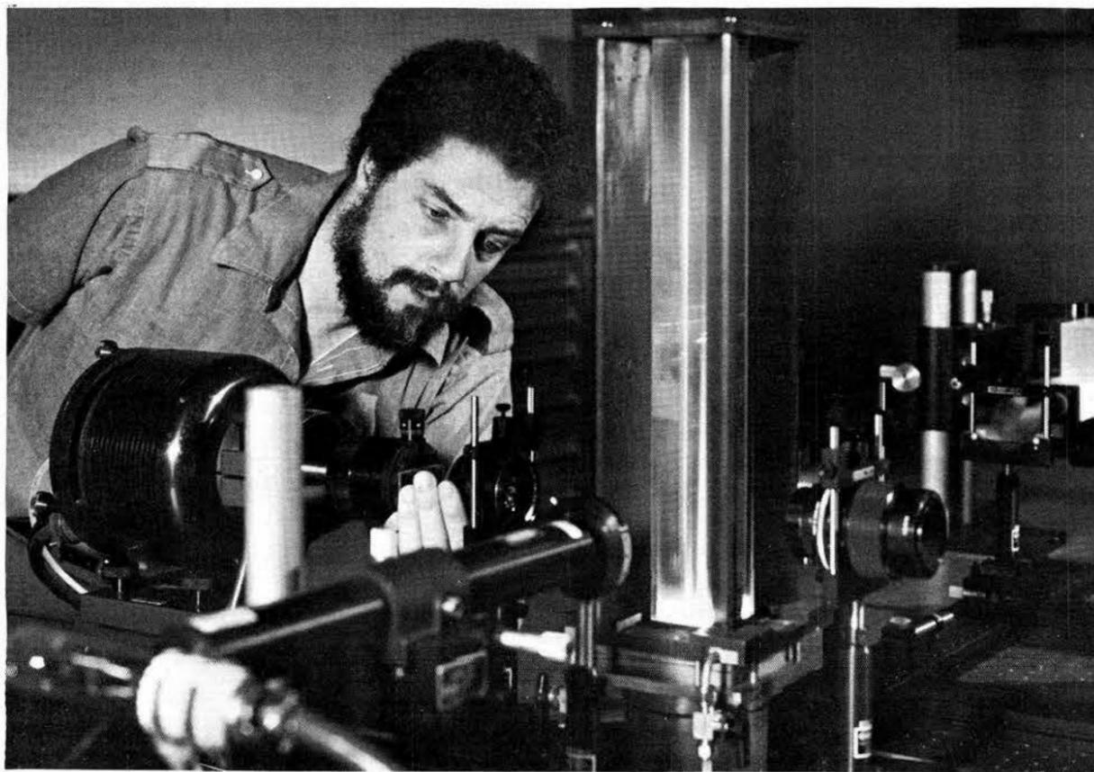
Bill McLean (8353) notes the evolution of the coal combustion process in a combustion-driven flow reactor.
