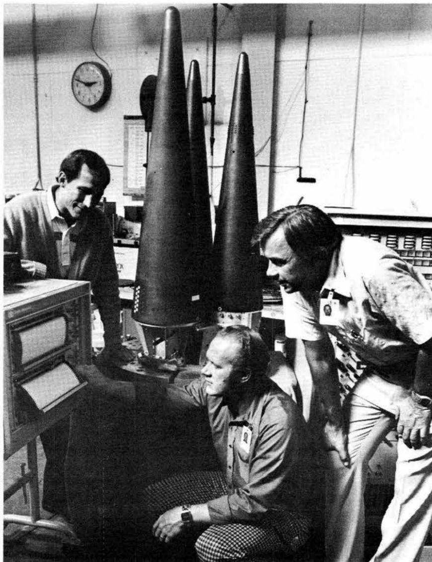
THREE SMALL RE-ENTRY vehicles, scaled in size and weight to duplicate the performance of full-scale RVs, are checked out by (left to right) Bob Stearley, Marlyn Sterk and Ron Johnson, all of Exploratory Systems Division 5623. Each RV carries a number of weapon components and systems of different designs and materials. By launching all three aboard the same missile and exposing all three RVs to exactly the same environmental conditions, an entire test series can be run at one time.
