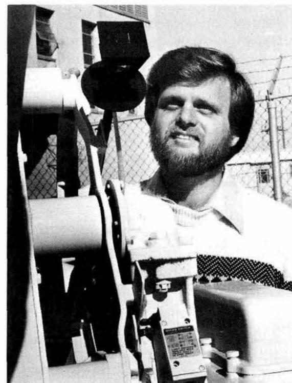
INVENTOR Gene Hammons (5132) examines his recently patented solar tracking device. Differences in the voltage of nine photovoltaic cells are used to control drive motors to position a solar collector. The collector is properly oriented when voltages in the tracking device cells are equalized.
