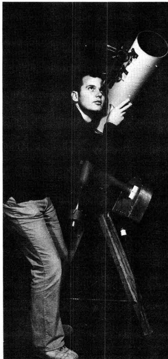
**BILL WAMPLER zeroes in on a deep-sky object with his 6-inch Newtonian reflector. He built the telescope when he was in high school—the instrument has an equatorial mount and clock drive.**
