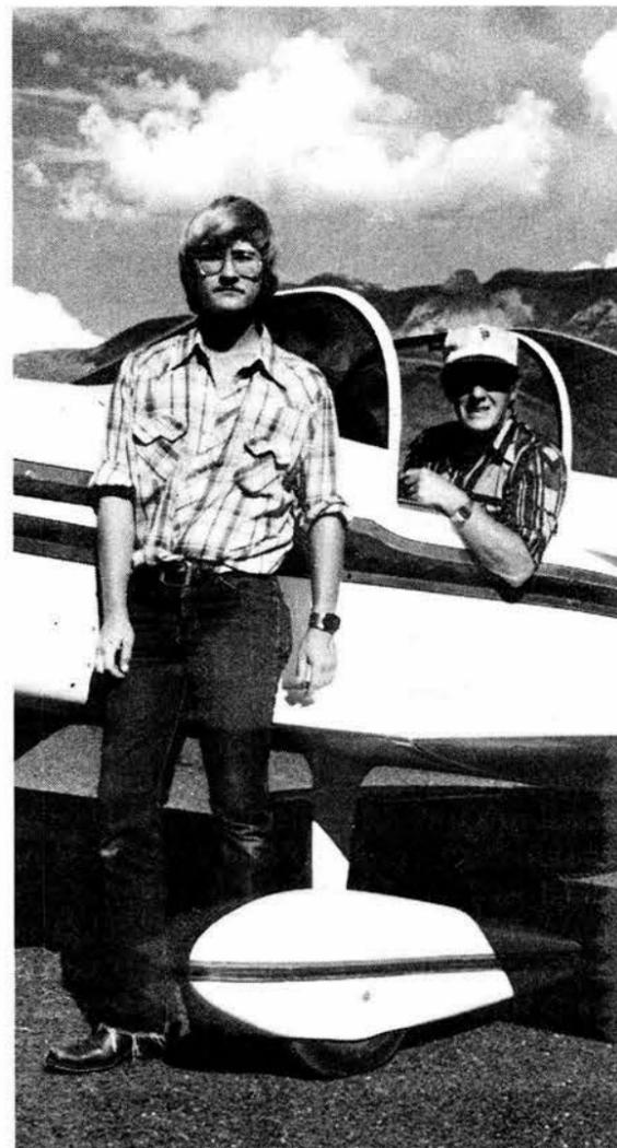
BILL GUERNSEY (1481), in cockpit, and his son Billy spent 12 years building this all-metal Mustang II. Billy was six when he started helping with the project. Completed in September, the plane has top speed of 250 mph and a 1700-feet-per-minute rate of climb with its 160 hp Lycoming engine. Pilot and passenger sit side-by-side in plush custom interior.
