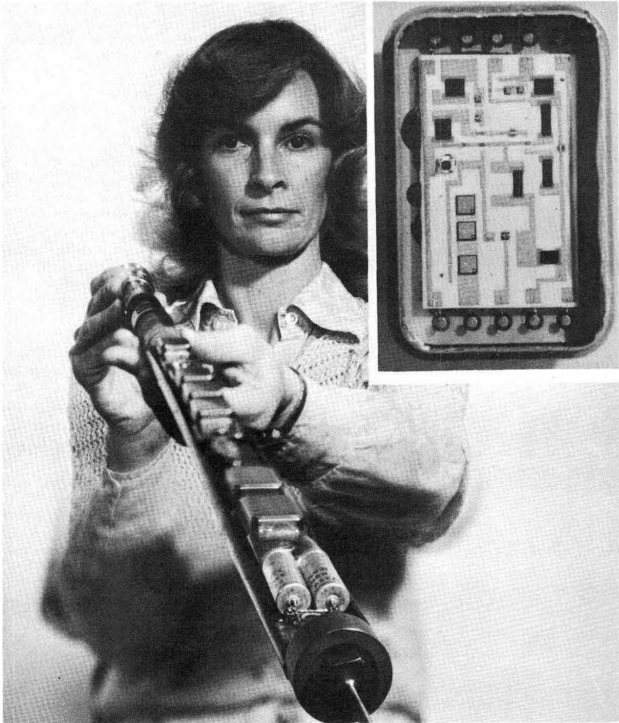
PEGGY BONN, an ESA in Geothermal Technology Division 4742, holds the complete electronics package used in the geothermal well temperature tool developed by Sandia. The tool is equipped with electronic microcircuits that operate at 275°C. These microcircuits, under development at the Labs for the past four years, are now commercially available.
