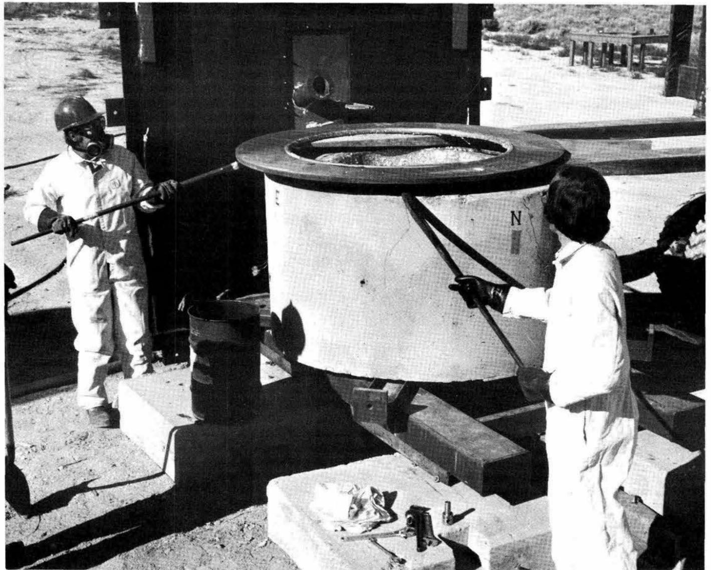
WHAT HAPPENS when molten sodium is spilled on tests simulating molten sodium spills were run with concrete is a reactor accident scenario under investigation in Advanced Reactor Research Dept. 4420. In 1980, several concrete containers like this.
