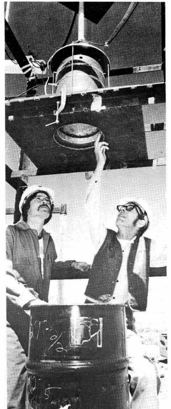
IN OPEN GEOMETRY a crucible (above) is readied for a steam explosion experiment in Area Y by Walt Nickerson and Carl James (both Ktech Corp.). The graphite crucible is designed to deliver the melt as a coherent mass into the water chamber.
