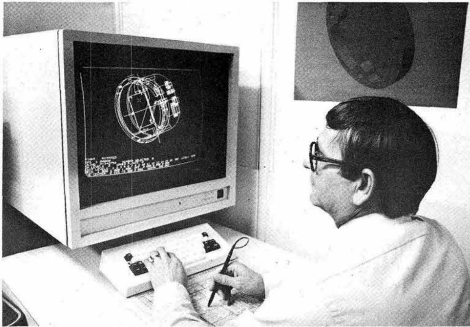
WADE ADKINS (2454) calls up a model of the W85 Joint Assembly from the CAD graphics files. The complete system or any component may be displayed, from any angle and to various scales. CAD is particularly valuable in the early stages of design and is now the first link in the automated production of machined parts.
