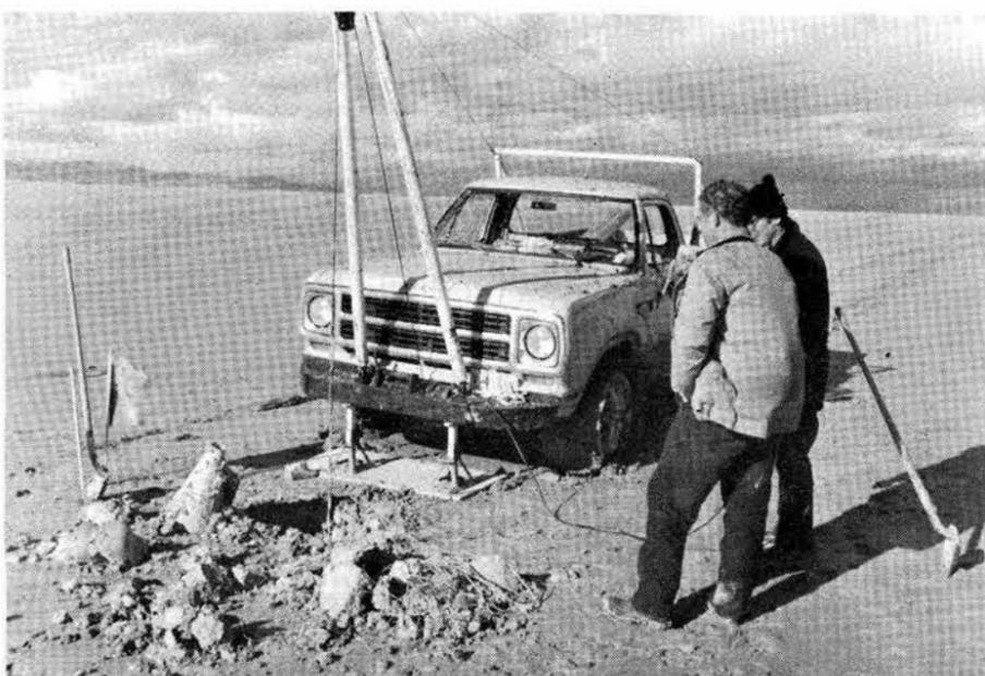
RETRIEVING sheared-off tail section, Wayne Young and Bill Jacoby contemplate tenacity of mud. Sample of mud tested in laboratory froze only when temperature was lowered to 5°F because of high salinity.
