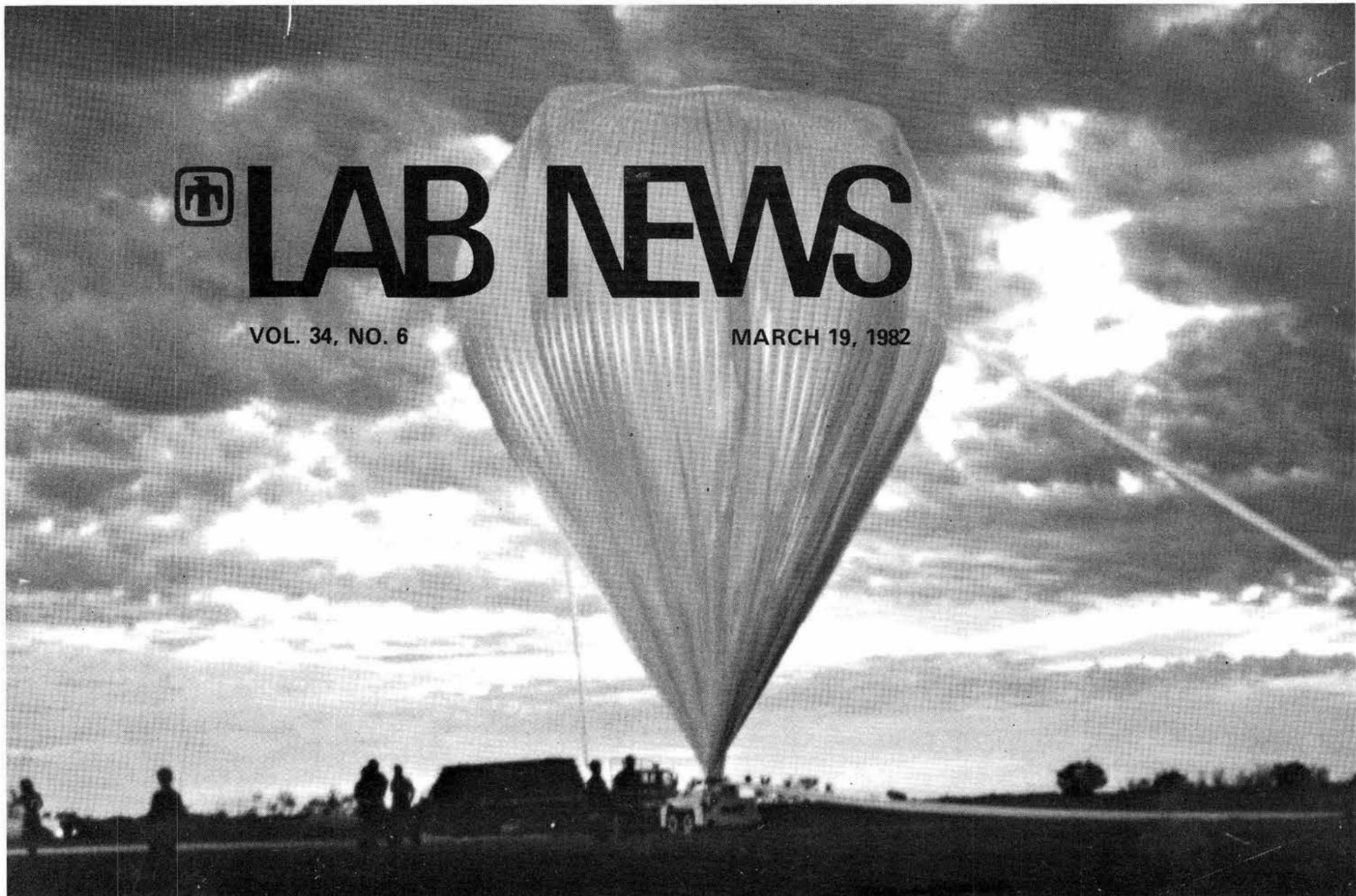
PARTIALLY INFLATED with helium, the experimental balloon stands poised for a dawn launching. When inflated, the 20.5-million-cubic-foot balloon rose to
