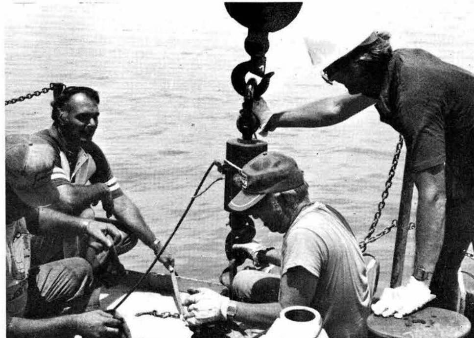
GETTING DOWN to the work at hand—attaching a load-cell to the line used for recovery of the ISP-2 telemetry package—are Jack Bahlman, Ray Wood, Jim Gallagher, and project leader Tom James.
