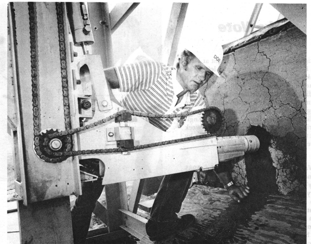
DOWN AND OUT is how this new drill operates in order to drill a horizontal shaft from the bottom of vertical drillhole. Project leader Dave Shirey (9747) checks the cornering mechanism as the drill starts into a test block of simulated coal.
