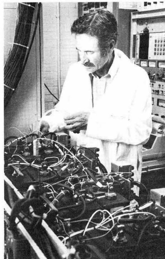
DON BUSH (2525) prepares apparatus for deep-discharge cycling test of a new battery developed for solar energy applications. Almost 700 cycles have been completed on some batteries with only modest loss of energy storage capacity.
