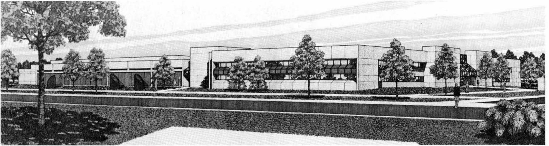
CONCEPTUAL DESIGN of the new VLSI facility for the 2100 organization is part of the package of design specifications prepared by Mike DeWitte's Buildings and Facilities Design Division III 3643. The two-story building will have two separate but related sections — an office and light laboratory area and a 13,000-square-foot "super" clean room (Class 1-10 clean room — less than one micro-
