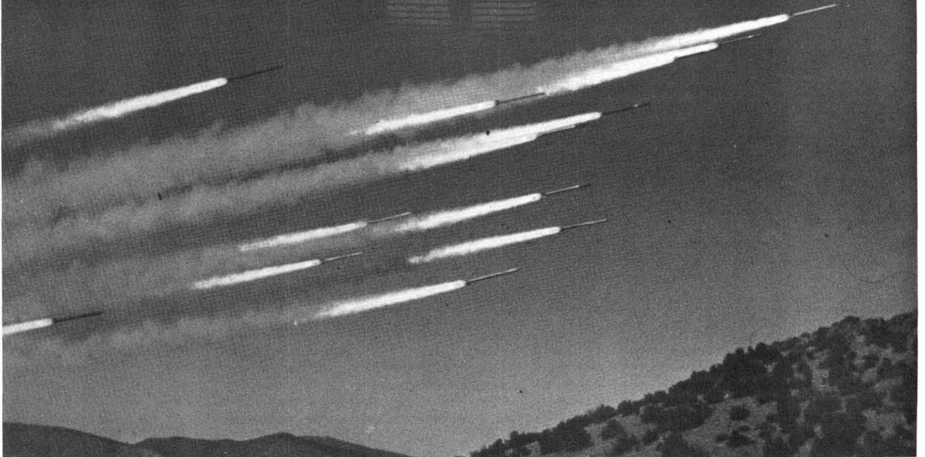
THIRTEEN-ROCKET SALVO above flies toward a target with no significant interference among the rockets. Before the launch (right), the rockets were arranged in a concentric cluster. A computer model of trajectories led to a firing sequence that minimized in-flight interference but allowed all 13 to strike the target simultaneously.
