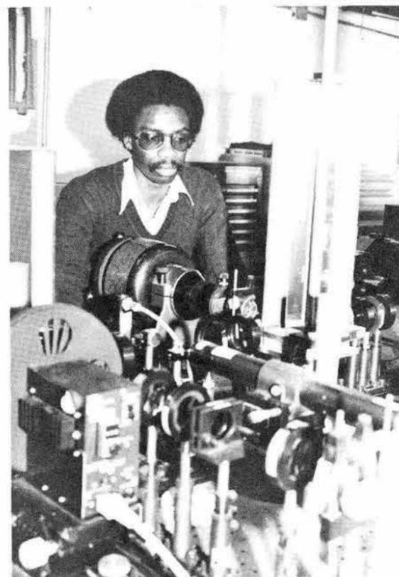
IN COAL LAB, Reggie Mitchell (8521) experiments with coal and other pulverized fuels to find ways of burning them more efficiently. Reggie has devised a new technique to measure a single particle's temperature while it is reacting.
