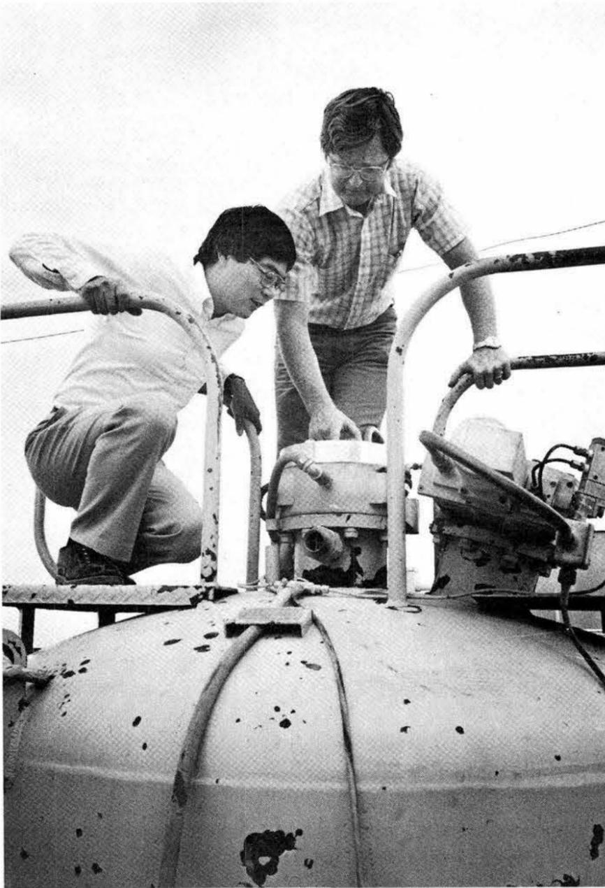
CLAMBERING on top of the furnace at the Large-scale Melt Facility are T.Y. Chu and John Bentz (both 7537). The IMF, the world's largest facility of its kind, permits researchers to investigate, on a scale and at temperatures never before possible, the safety-related phenomena that would occur if a reactor core-cooling system were to fail.
