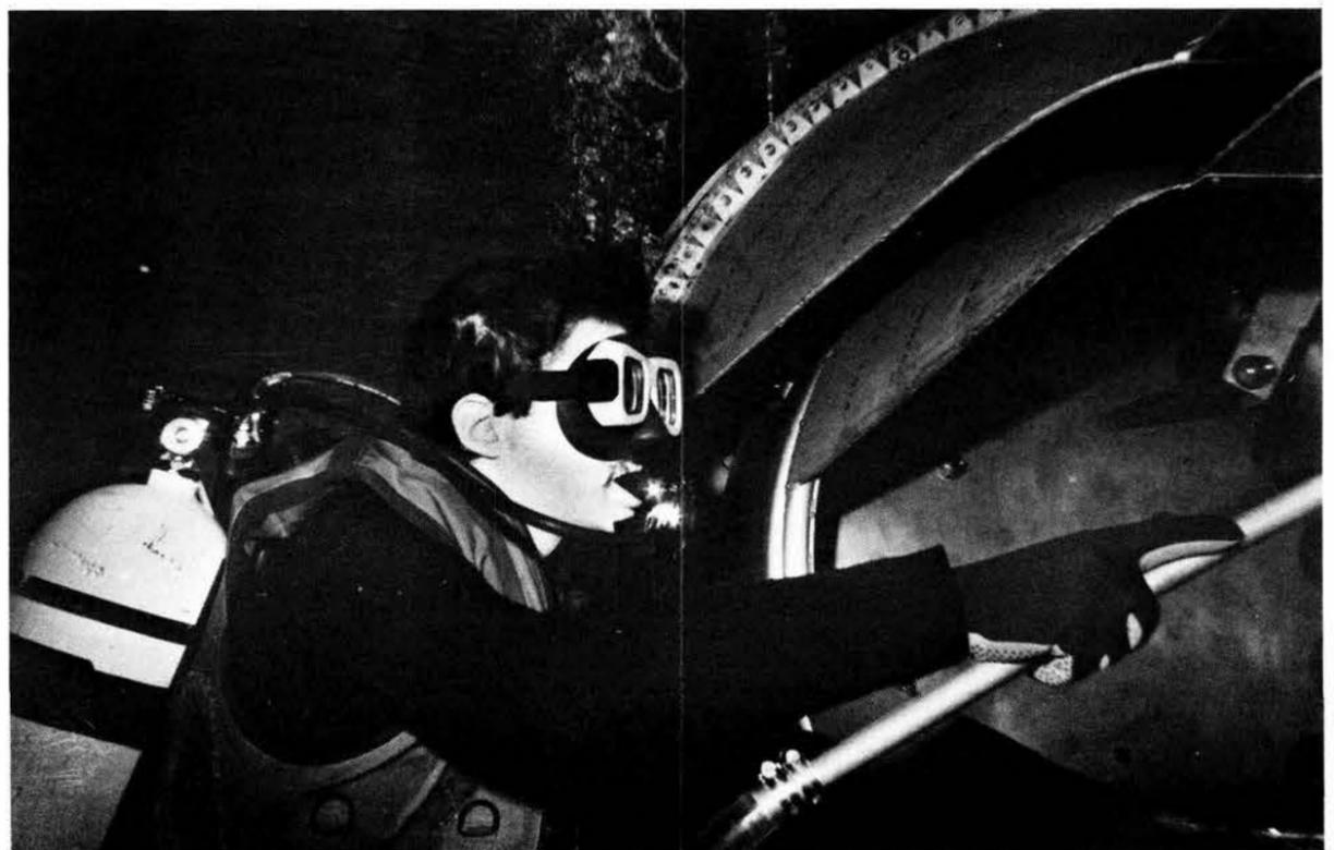
IN-DEPTH TECHNOLOGY — Richard Cleary of K-Tech and his SCUBA gear remove bubbles from the transition section of a PBFA-II module now being tested in the Demon facility in Area IV. (Underwater photography by Mike Eaton, K-Tech)
