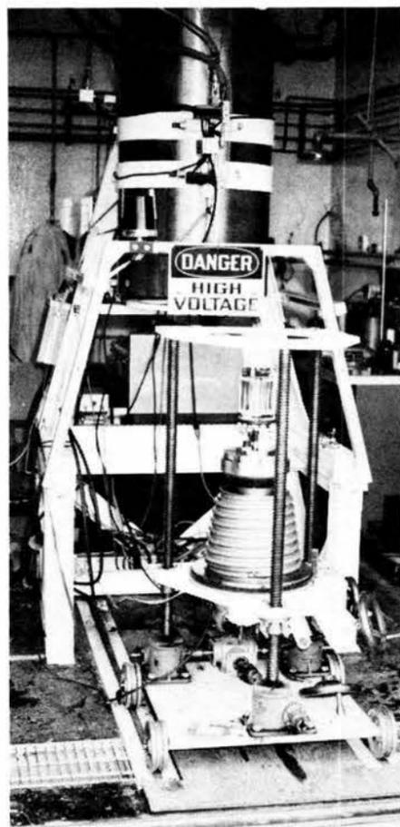
MAGMA SIMULATION FACILITY allowed the first direct measurements of heat transfer rates in a basaltic magma under typical magma chamber conditions.
