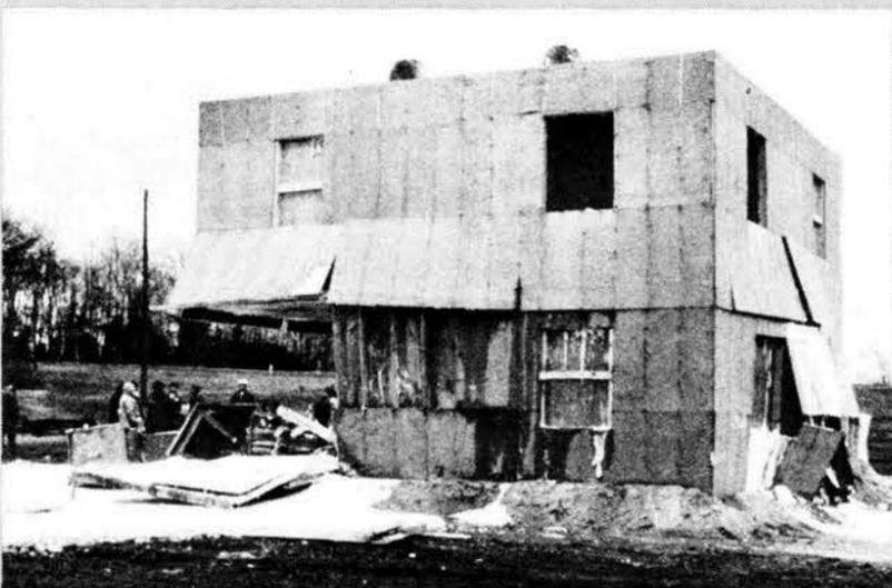
DRAMATIC BLAST MITIGATION effect of aqueous foam is illustrated in these two photos taken during a joint study by Sandia's Special Projects Division 5256 and the Naval Tech Center's Explosive Ordnance Disposal group at Indianhead, Maryland. In the photo at left, a two-story frame test structure was filled with aqueous foam, then 15 lbs. of C4
